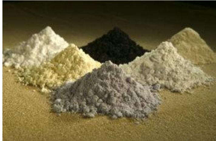
In this undated photo released by the U.S. Department of Agriculture are rare-earth oxides, clockwise from top center: praseodymium, cerium, lanthanum, neodymium, samarium, and gadolinium.
